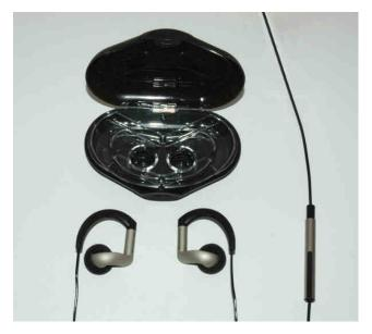
Fortunately, the carrying case is easy to use as the left and right earpieces fit into an inner hinged plastic holder with a moulding to wrap the wires around. The 'stick' volume control is neatly positioned along the wire so that it lines up nicely with its slot in the holder. The volume control itself incorporates a sliding shaft to adjust the volume – very elegant and, dare I say, stylish?
