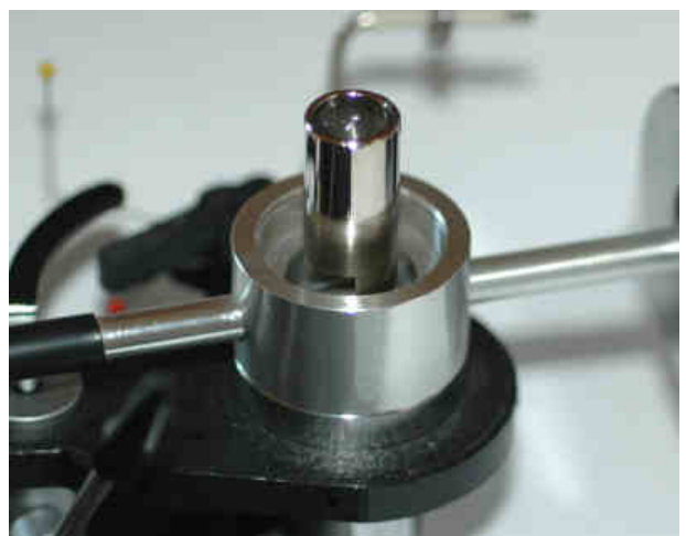
Figure 9. Close-Up of Dashpot
