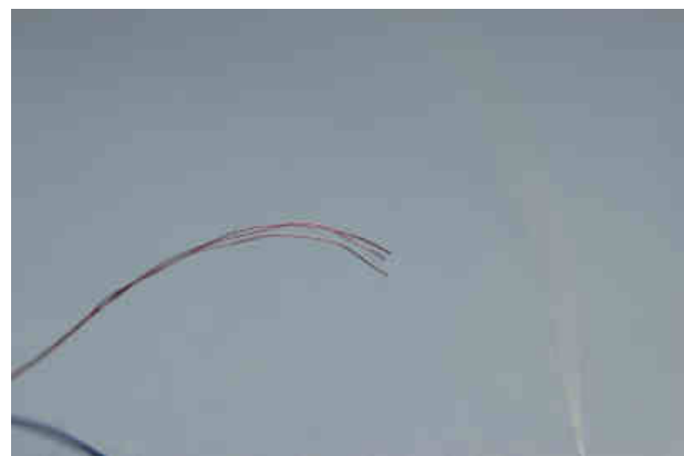
Figure 4. Close-up of Red Wire Showing the Three Strands
