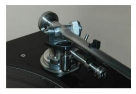
sounds clear. To cater for us 'tweakers', there are several solutions out there in the form of VTA adjusters for the older RB250, RB300 and RB600, such as the Michell Engineering VTA Adjuster. However, the only company I am aware of that makes adjusters for the entire current range of Rega 3 point fixing arms is ISOkinetik. These are of a particularly high quality and one was fitted to the arm being tested.
