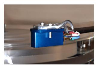
The first parameter to check was the tracking ability using my copy of the Vinyl Essentials test record. This confirmed the quoted figure by tracking the 80 microns test track but failed on the 90 micron track. This is a pretty good figure in any case and was an improvement on the Lyra, which could only just manage 70 microns.
