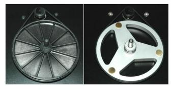
The ISOsub sub-platter kit comprises a replacement phosphor-bronze bearing supplied with either a ruby (as reviewed here) or ceramic 4.7mm diameter ball, together with an aluminium and ground-steel sub-platter assembly. The sub-platter is precision engineered with 0.001mm concentricity between the axle and hub. This greatly improves pitch control and should add grip to the lower and sub frequency ranges. The ISOsub is supplied together with some "ISOlube" long chain carbon spindle oil.
