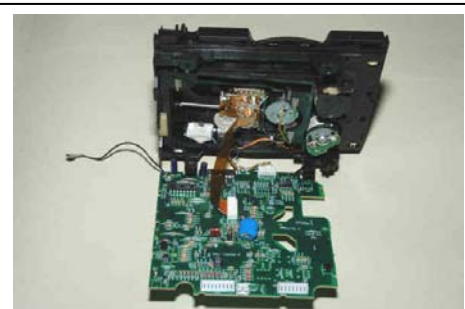
Removing the drive circuit board
