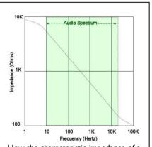
How the characteristic impedance of a typical 75 ohm coaxial cable varies with frequency, with the greatest changes occurring within the audio spectrum!
