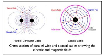
Not only are the choices of material important in the design of cables, but also in their construction. Coaxial cables have the benefit of containing the electric and magnetic fields within the cable and help to screen out interference from outside sources and are therefore the design of choice for audio interconnects. Mains and loudspeaker cable construction ranges from simple parallel wires to complex weaves of individually insulated wires.
