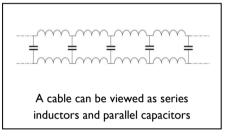
voltage (and capacitance has the inverse effect), cables will cause minute phase errors between current and voltage which are frequency-dependent.
