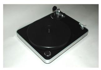
The Concept is equipped with a new tonearm that incorporates a friction-free magnetic bearing and is fitted with a high quality Clearaudio Concept moving magnet cartridge. Apart from low friction, the magnetic bearing allows the arm to be shipped with the counterbalance weight and cartridge installed without risk of damage to the arm bearing. All the necessary adjustments are already completed at the Clearaudio factory - even the tracking weight and anti-skating force are pre-adjusted.
