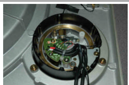
Old arm base ready for removal
