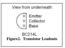
The input from the cartridge is delivered to the emitter of the BC214L via a coupling capacitor, C3. C2 ensures no RF finds its way into the system. The input impedance of the amplifier is about  $200\Omega$  with a load capacitance of 6.8nF, which should suit most moving coil cartridges. If a higher load capacitance is required, then an appropriate value can be strapped across C2.
