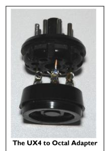
Use a thick solid copper wire to ensure that the final assembly is rigid and will hold the 300B firmly without any tendency to flop over!
